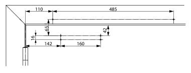
Fitting dimensions with mounting plate for standard installation on hinge side
