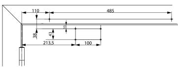
Fitting dimensions for direct standard installation on hinge side
