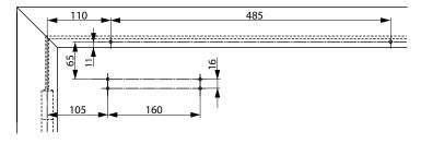
Fitting dimensions with mounting plate for standard installation non-hinge side
