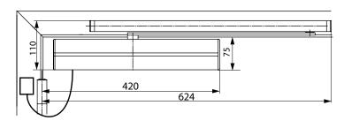
Regular door mounting Left hand door shown in diagram Right hand door is the reverse
