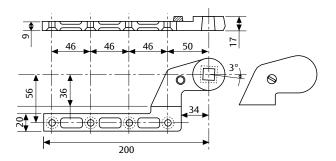
Right bottom arm in steel for single action doors, 36mm. offset. Square French spindle. Silver painted ABS covers.
