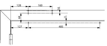
Fitting dimension for standard installations on hinge side frame mounting with guide rail
