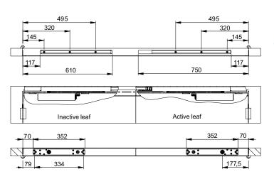
Installation dimensions with 8 mm spindle extension
