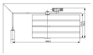
Regular door mounting Left hand door shown in diagram Right hand door is the reverse
