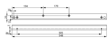
Angle bracket A116 For guide rail G460 nonhinge side installations
