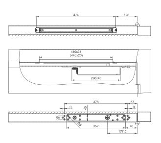
**Installation dimensions** with 8 mm spindle extension
