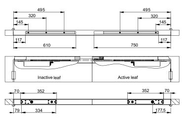
Installation dimensions with 8 mm spindle extension
