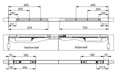
Installation dimensions with 4 mm spindle exten-
