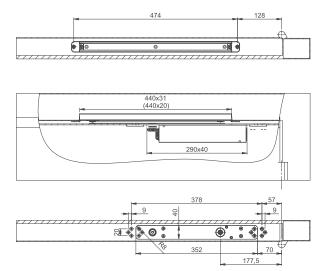
Installation dimension for standard door fitting Right hand door shown
