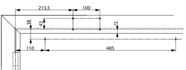
Fitting dimensions when mounted directly onto the grame hinge side
