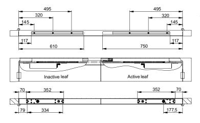
Installation dimension for standard door fitting Right hand door is active leaf Left hand door is inactive
