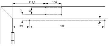
Fitting dimensions with mounting plate for frame mounting on hinge side
