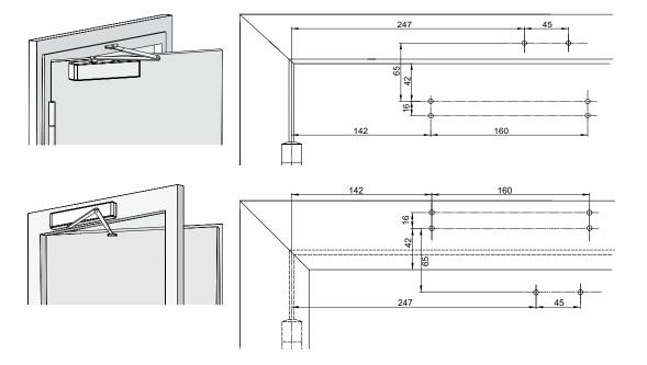
Fitting dimension for standard installations on hinge side with link arm Left hand door shown in
