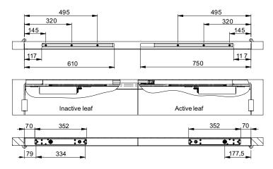
Installation dimensions with 4 mm spindle extension
