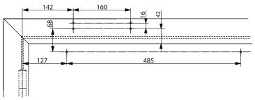
Fitting dimension for standard installations on non-hinge side with guide rail
