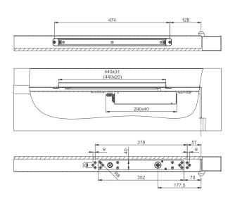
Installation dimensions with 4 mm spindle extension
