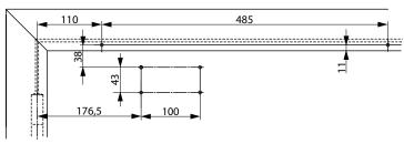
Fitting dimensions for direct standard installation non hinge side Right hand door shown in diagram
