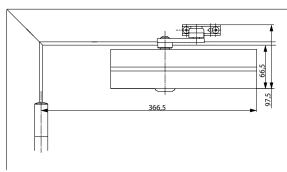
Regular door mounting Left hand door shown in diagram Right hand door is the reverse
