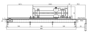
Installation dimensions for top jamb application Right hand door shown in diagram
