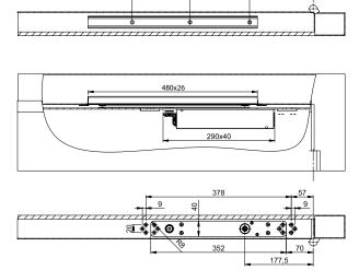
**Installation dimensions** with 4 mm spindle extension
