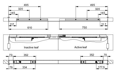
Installation dimensions with 4 mm spindle extension
