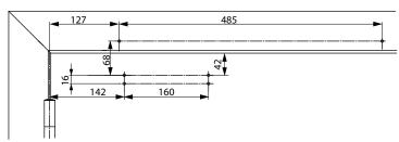
Fitting dimensions for standard installation on hinge side with guide rail Left hand door shown in diagram Right hand door is the
