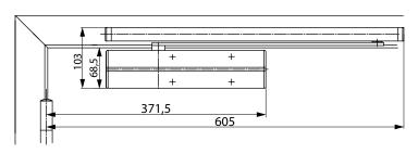
Space required on doors for standard installation on hinge side
