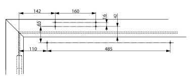
Fitting dimensions with mounting plate for frame mounting non-hinge side
