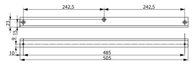
Angle bracket A104 Only for standard guide rail L694
