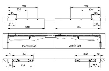
Installation dimensions with 8 mm spindle extension
