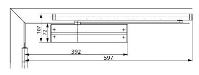
Regular door mounting Left hand door shown in diagram Right hand door is the reverse
