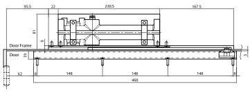
Installation dimensions for top jamb application Left hand door shown in diagram
