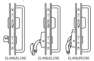
The lock is electrically controlled by access control system.
