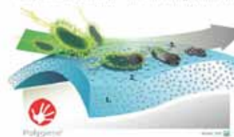
The silver is homogeneously distributed throughout the material. Silver migrates to the surface. Silver ions kills the bacteria on the surface by penetrating the cell membrane
