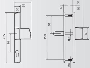
The profile door handles are used in aluminium and steel profile doors with a profile door lock and as an espagnolette handle in balcony doors.
