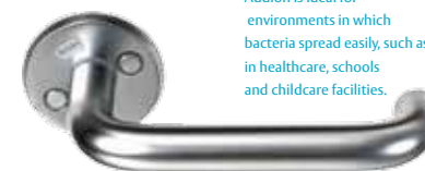
The silver is homogeneously distributed throughout the material. Silver migrates to the surface. Silver ions kills the bacteria on the surface by penetrating the cell membrane
