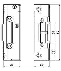
Minimal dimensions allow the electric strike to fit into the frame easily.
