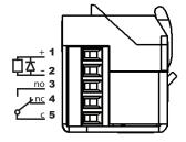
Connection takes place using a screw terminal block. Built-in protector diode.
