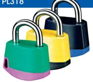
A multi-purpose padlock with 6,5 mm chrome plated steel shackle and diecasted lock body with coloured plastic cover. The options of colour for plastic cover are dark blue/light blue, green/violet and yellow/black. Cost effective product preferably for indoor use eg. cabinets and tool boxes.
