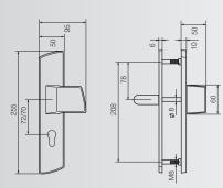
Also available as a profile door handle. The long plate is 30 mm wide in the profile door handles. Tested according to EN179 and approved for use on fire doors according to standard EN 1634-1.
